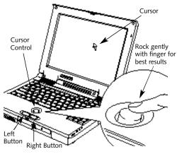
Figure 2-6 ErgoTrac Pointing Device
